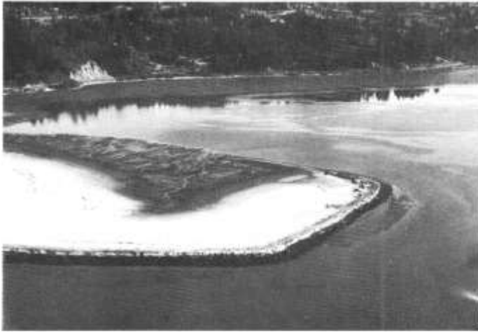
Figure 3. This tideland fill in Sallys Bend destroyed shellfish beds and altered current patterns in this area. Material eroded from the area covered stands of eelgrass and shellfish beds adjacent to the fill.
